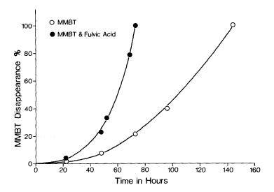
Figure 1. Enhanced MMBT biodegradation by FA in fermentor.
